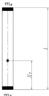
$$\begin{aligned} m_d &= m \frac{l - x_T}{l}, \\ m_d &= m \frac{x_T}{l}. \end{aligned} \quad (5.2)$$
