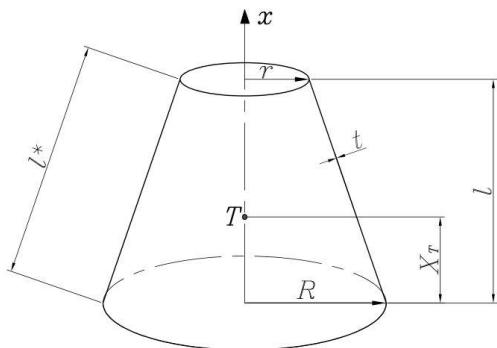
$$\begin{aligned} m &= \rho t \pi l^*(R + r), \\ l^* &= \sqrt{l^2 + (R + r)^2}, \\ x_T &= \frac{l}{3} \frac{R + 2r}{R + r}. \end{aligned} \quad (5.1)$$
