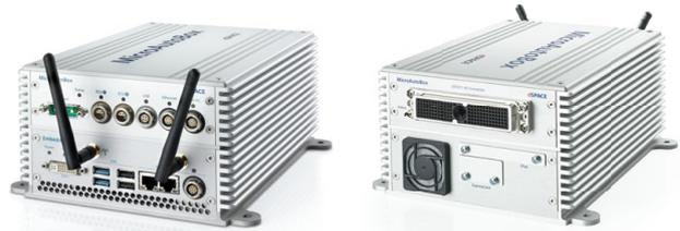
Example: MicroAutoBox II 1401/1511 with Embedded PC and optional WLAN module.
