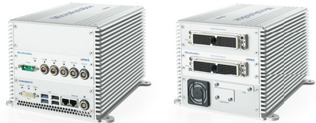
Example: MicroAutoBox II 1401/1513/1514 with Embedded PC.
