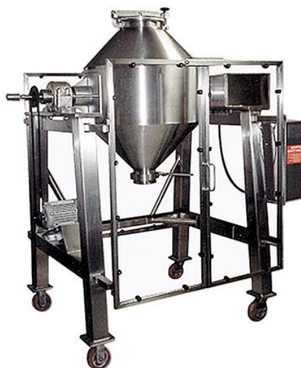
Sl. 3.10 Odabrani Double Cone prijenosni blender ACB30 (SERVOLIFT)
