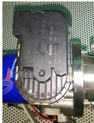
*Slika 4.19 Zaklopka snage Bosch PBT GF30*
