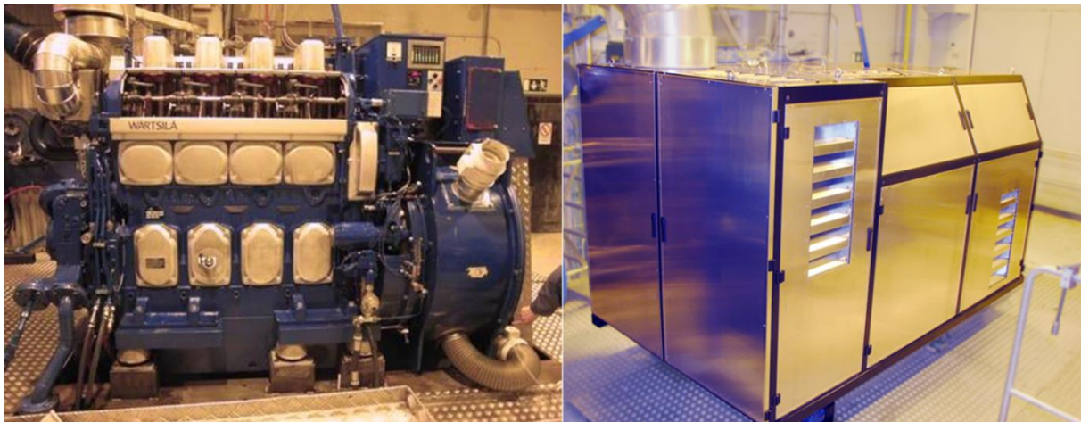
Figure 17 Wärtsilä's diesel engine without and with engine cover
