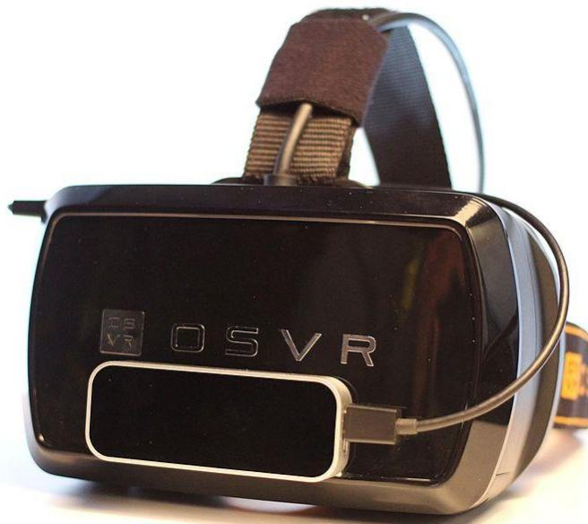
Slika 39. Kontroler Leap Motion montiran na OSVR headset [34]
