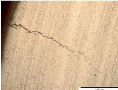
1000 µm              | Zavareni spoj napregnut vijkom<br>
