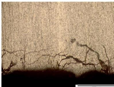
1000 µm        | Osnovni materijal napregnut vijkom<br>
