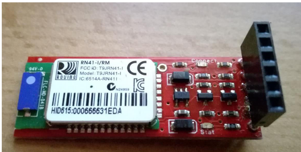
Slika 11. SparkFun Bluetooth Mate Gold modul
