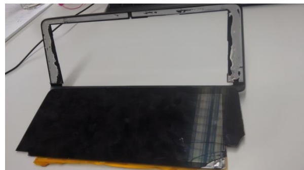
Visible tape on plastic frame after the cover glass is removed
