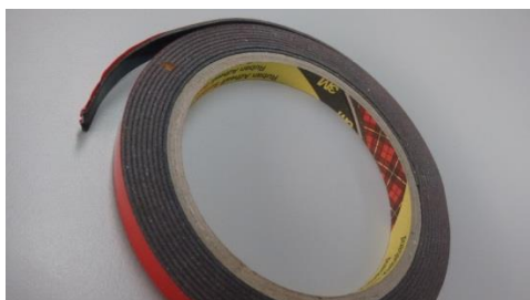
3M tape used for gluing the glass plate to the holder
