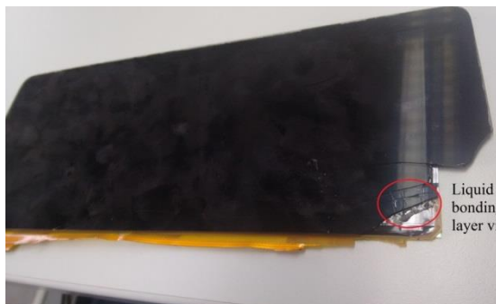
Separated LCD and cover glass from the plastic frame
