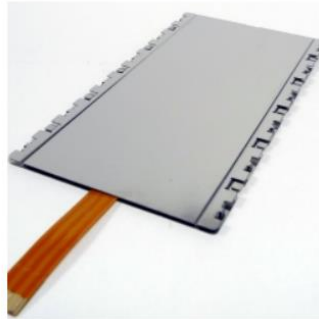
Figure 29. Reflex HIC Slide Actuator [Source: Artificial Muscle]
