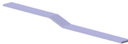
Figure 74. CAD model of the Z-shaped spring
