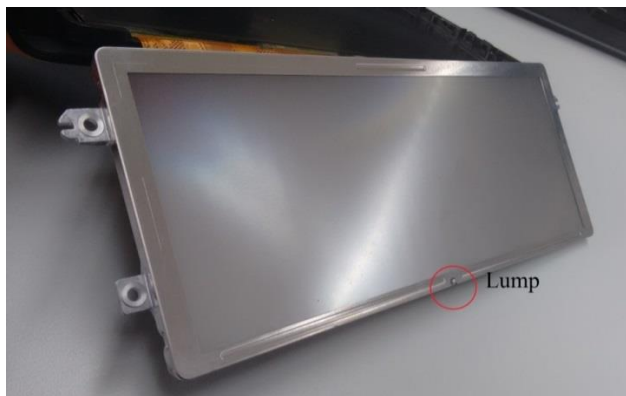
Separated backlight (used for the prototype)
