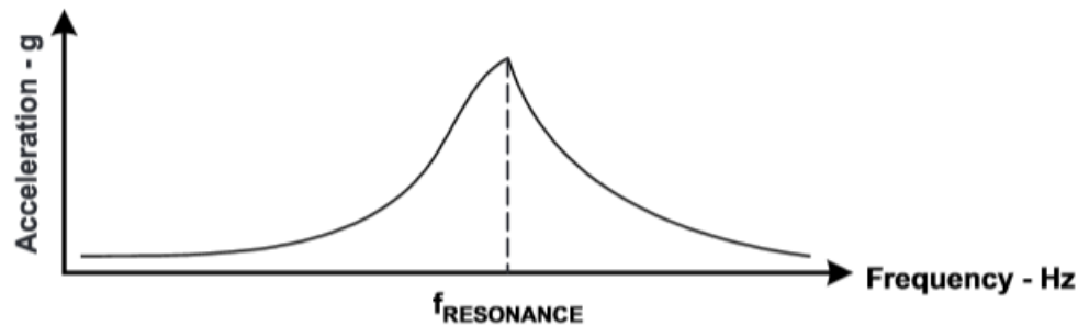
Figure 16. Typical LRA Response [30]
