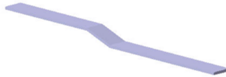
Figure 74. CAD model of the Z-shaped spring
