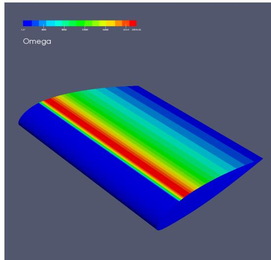
(b) Specifična disipacija  $\omega$ ,
