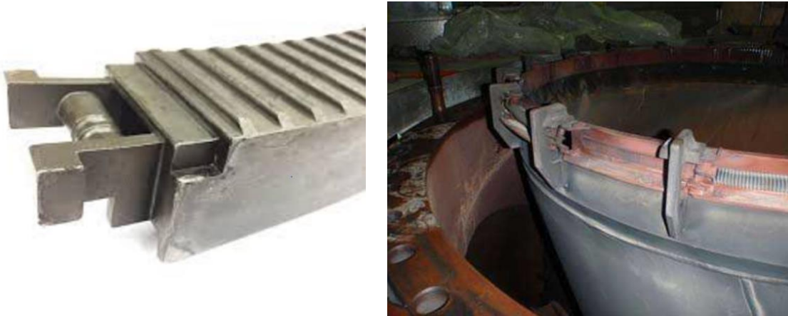
Figure 6. Segment of belt seal and belt seal mounted on Hot Gas Casing
