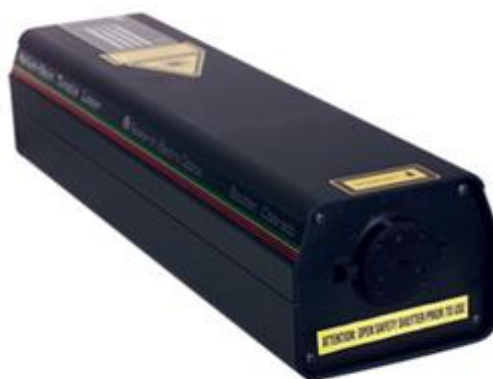
Slika 60. HTPS-EC Tunable HeNe Laser [26]
