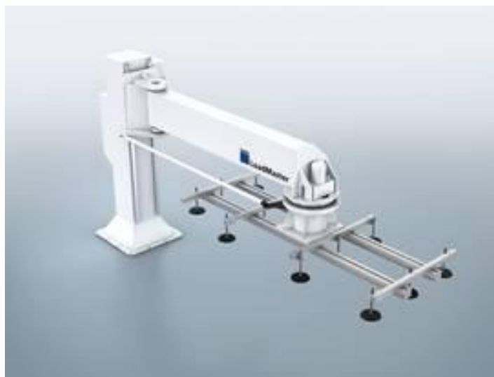
Slika 17. LoadMaster, Trumpf Automation [9]
