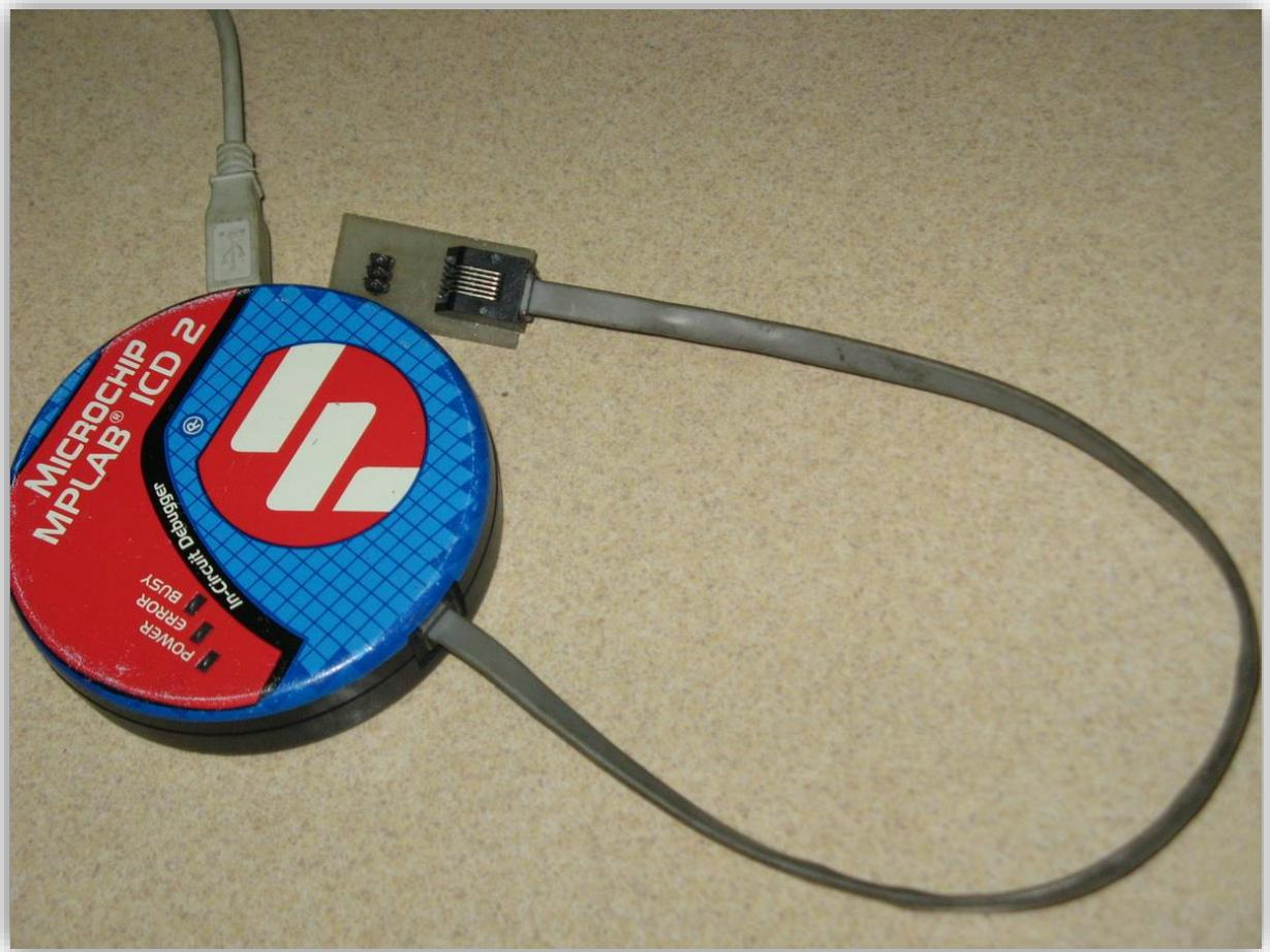
Slika 2. MPLAB ICD 2 programator [8]
