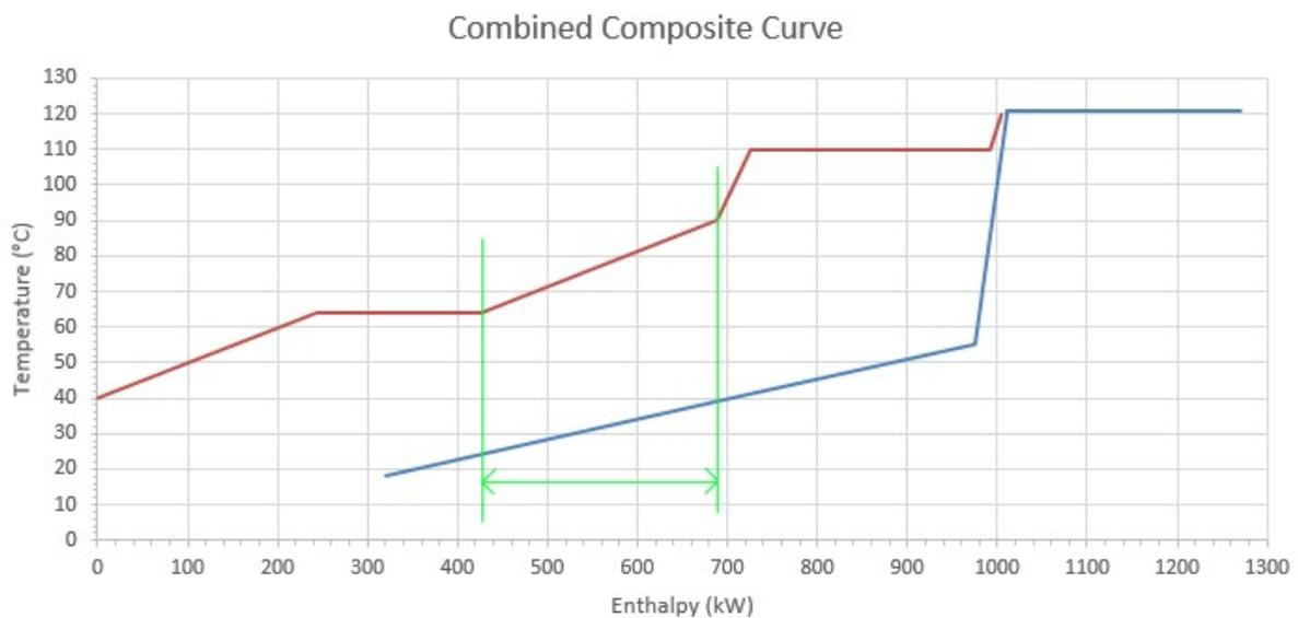
**Figure 7** Example of one enthalpy interval
