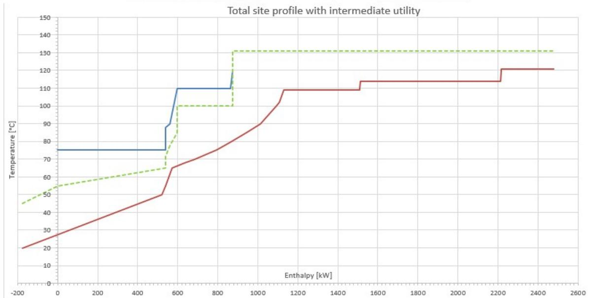
Figure 25 Final Total site profile with intermediate utility
