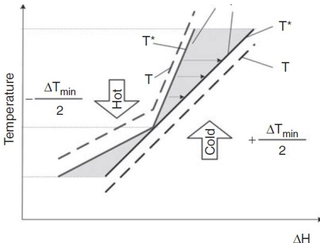
Figure 3 Shifting temperature [1]
