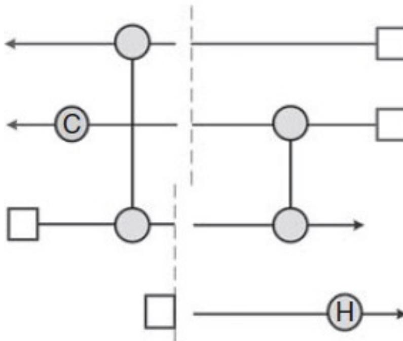
Figure 8 Simple representation of HEN grid diagram [1]
