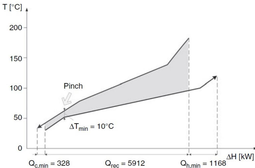
Figure 2 Pinch point for  $\Delta T_{\min} = 10^{\circ}\text{C}$  [1]
