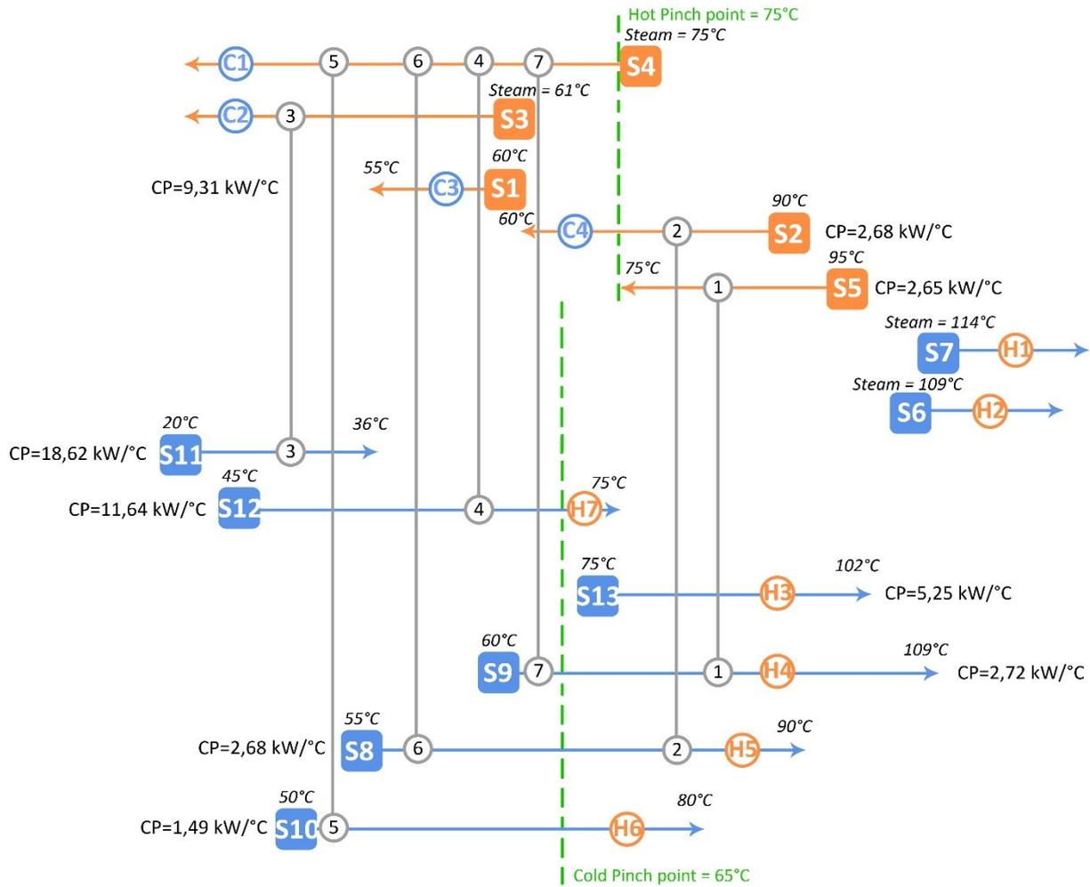
Figure 20 HEN network grid diagram (Process B)
