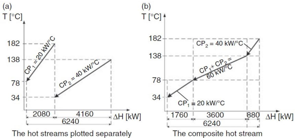
Figure 1 The construction of hot composite curve [1]
