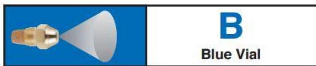
SOLID-CONE Type B-nozzles produce a spray that distributes droplets fairly uniformly throughout the complete pattern. The spray pattern becomes progressively more hollow at higher flow rates, particularly above 8.00 GPH. Provides smooth ignition and efficient combustion, particularly in larger burners.
