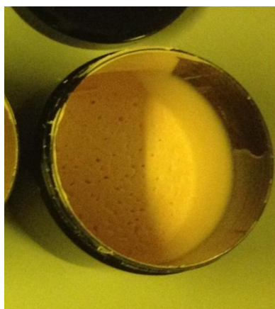
Figure 24. Separation of components in the slurry
