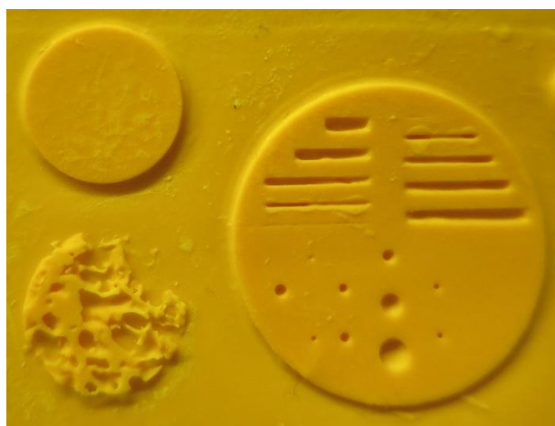
Figure 38. Printing quality of the slurry containing M3 and M5, with wax-solvent ratio of 20 wt% - 80 wt%
