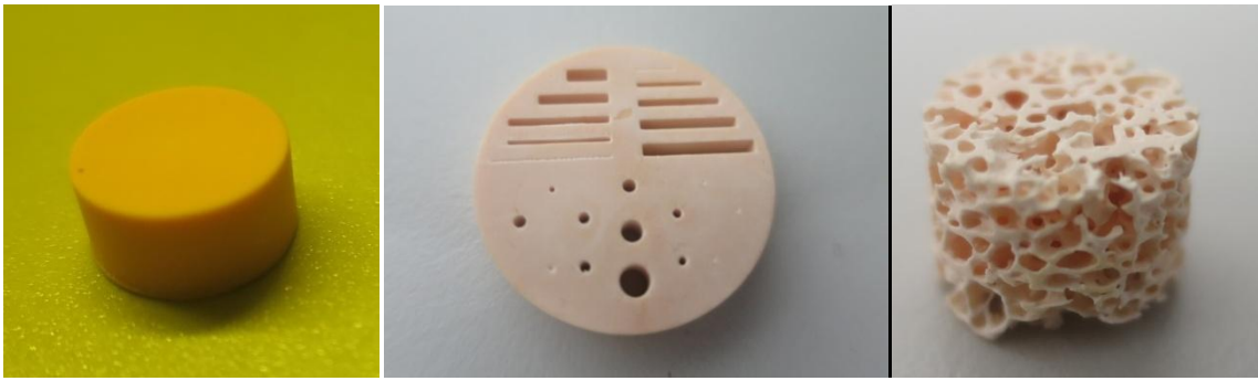
Figure 15. Structures used for testing of the printing quality
