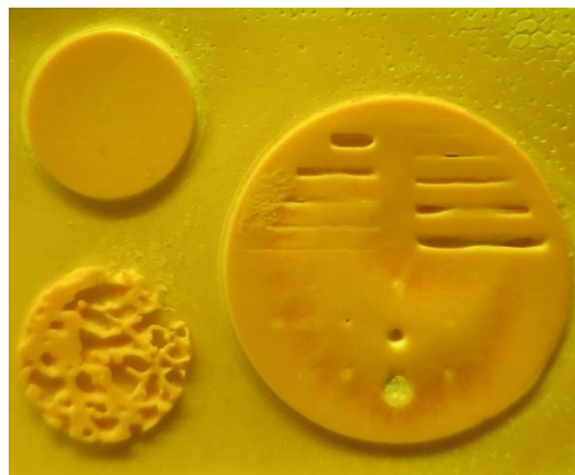
Figure 49. Printing quality of the slurry with D4 (light intensity: 63 mW/cm 2 )
