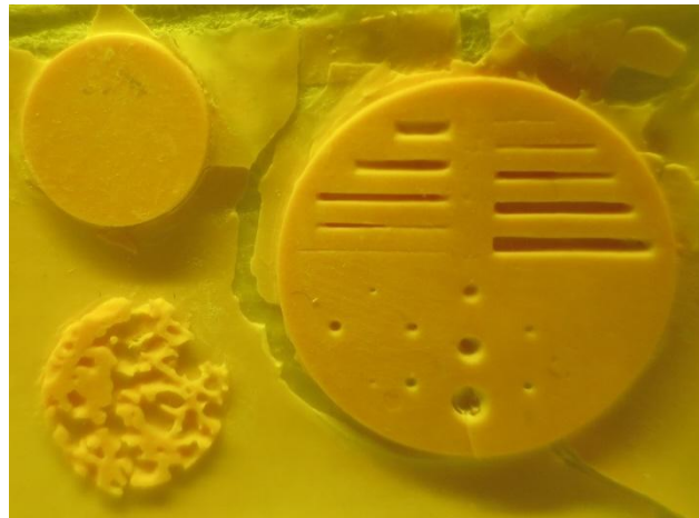
Figure 41. Printing quality of the slurry with 5 wt% increase in monomer content and wax-solvent ratio of 40 wt%-60 wt%
