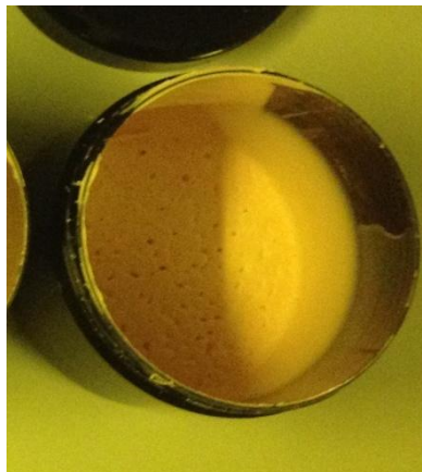
Figure 24. Separation of components in the slurry
