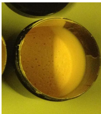
Figure 24. Separation of components in the slurry
