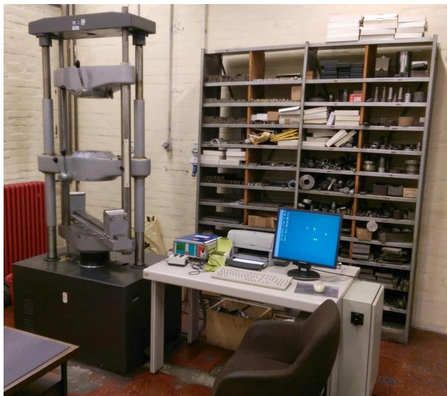
Slika 5.15. Kidalica WPM Heckert 400kN
