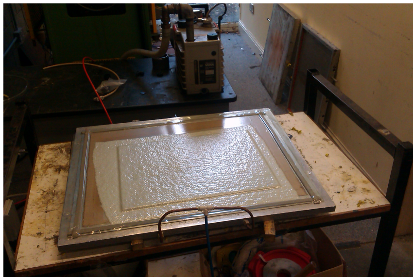
Figure 2.2: Debulking vacuum check
