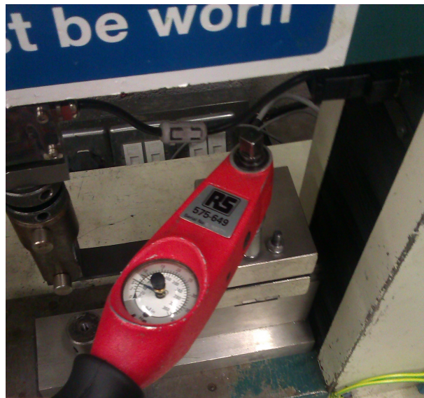
Figure 3.2: Tightening of the clamp using a torque wrench
