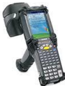
Figure 10-3 RFID reader system
