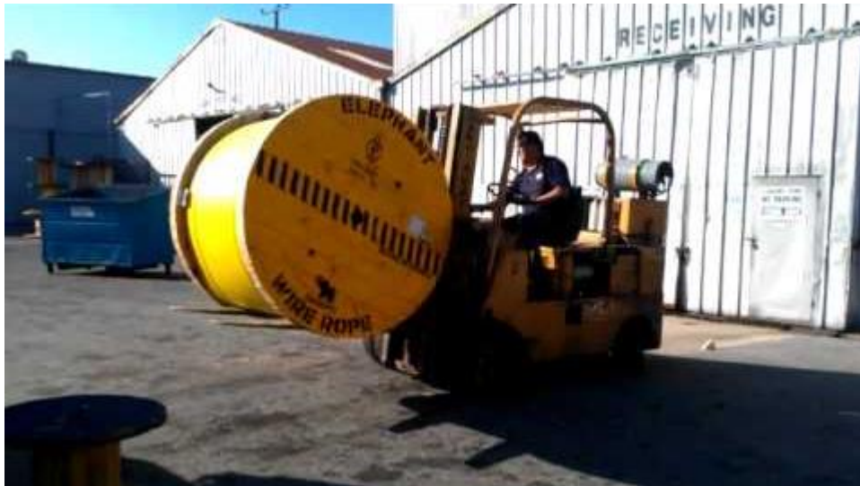
Figure 45. Forklift for spools transportation
