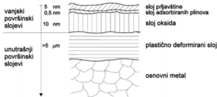
Slika 17: Shmaltz-ov model strukture rubnog sloja bez prevlake [15].
