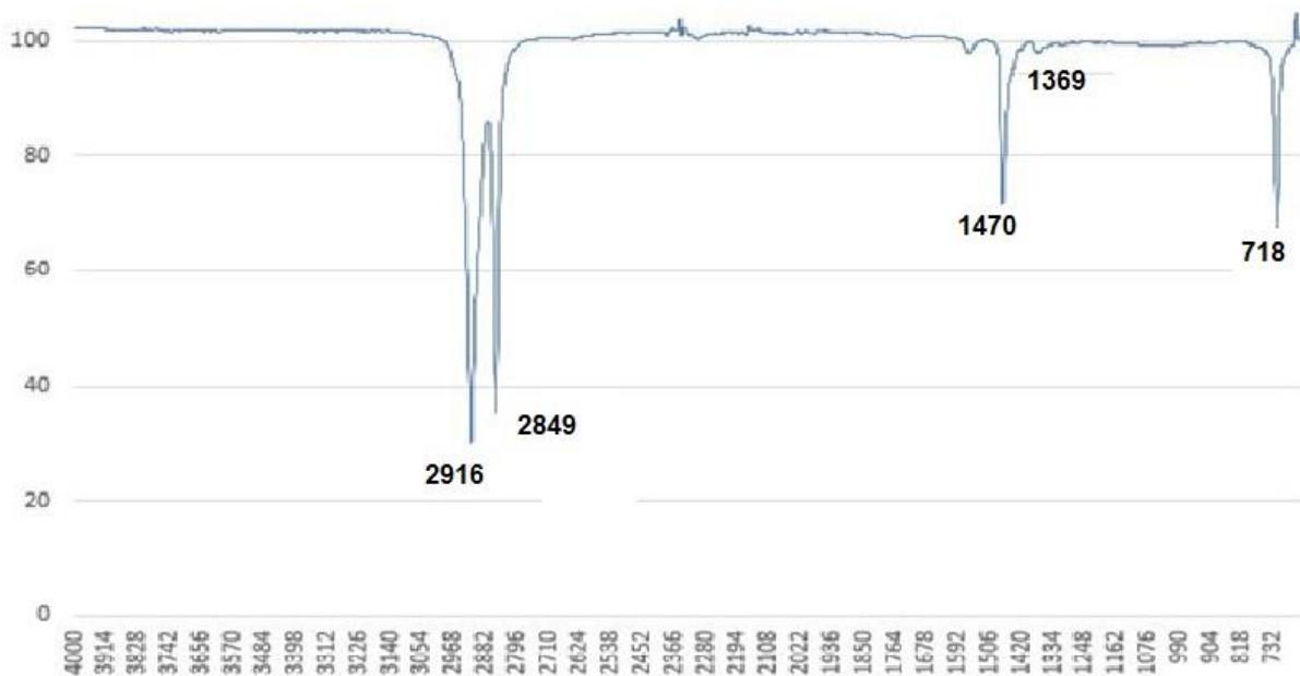
Slika 49. FTIR spektar folije od 100  $\mu\text{m}$  sa stane inhibitora
