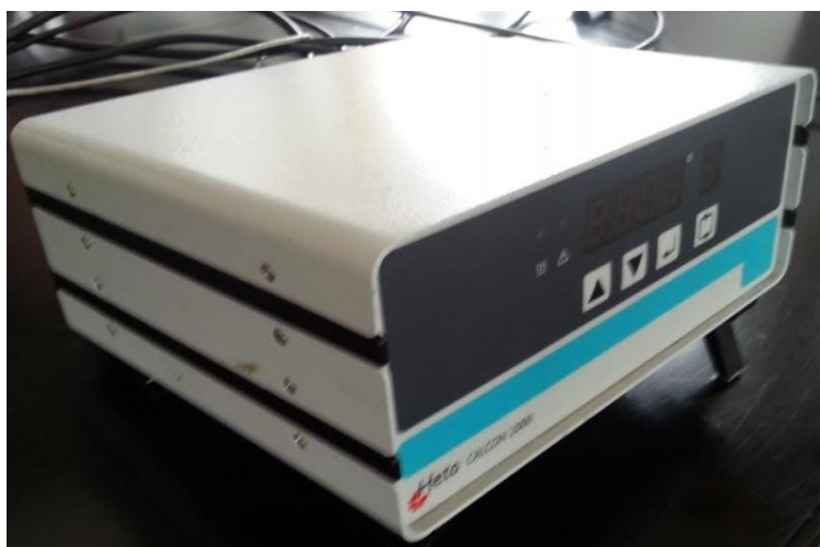
Slika 6. Calcon 2000, regulator temperature
