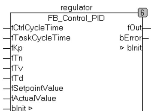
**Slika 6.2** *Pid regulator u CFC prikazu*
