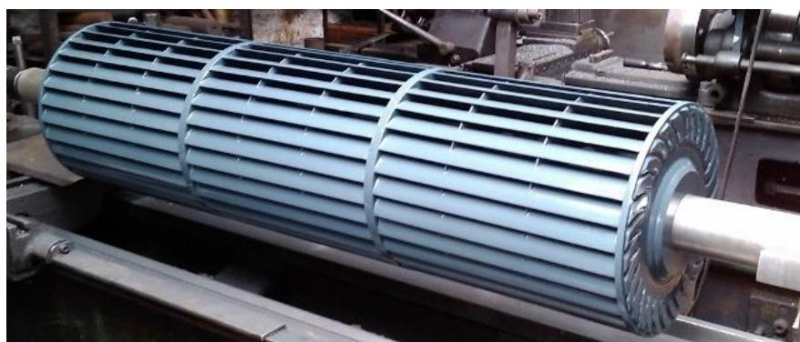
Slika 1 Rotor Ossberger turbine[1]
