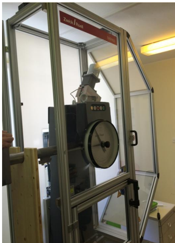
Slika 35. Instrumentirani Charpy-ev bat, ZWICK/ROELL, RPK 450
