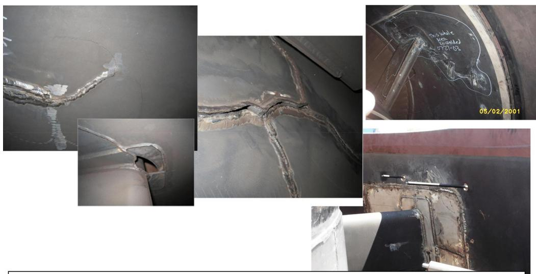
*Extensive Cracking seen in the inner and outer liners*
