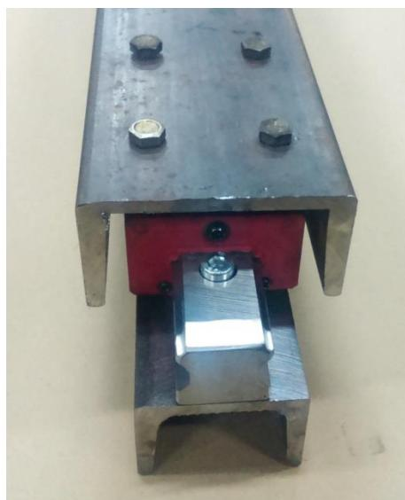
Slika 32: Sklop profila i linearne vodilice
