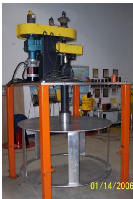
Slika 9. EnCurrent Squirrel cage Darrieusova turbina [4]
