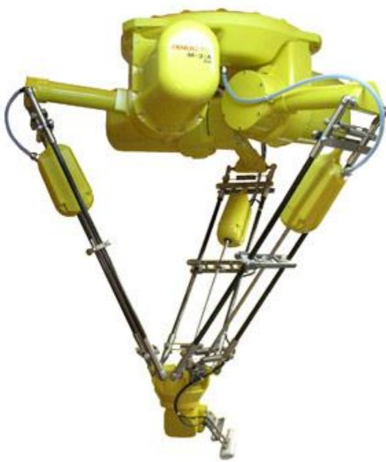
Slika 1 Robot FANUC M3iA/6a
