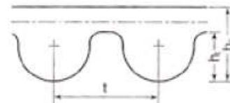
All M.E.C. TIMING BELT HTD and STD belts have a ground outside surface and a special fibreglass insert to □ ensure fluid movement.
