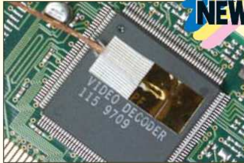
The self-adhesive mounting strip is ideal for "targeted" placement of the sensor element. Once the element is in place, it can be used "as is", for applications such as electronic component temperature monitoring during board fabrication. It can also be cemented in place using OMEGABOND® for higher temperatures.
