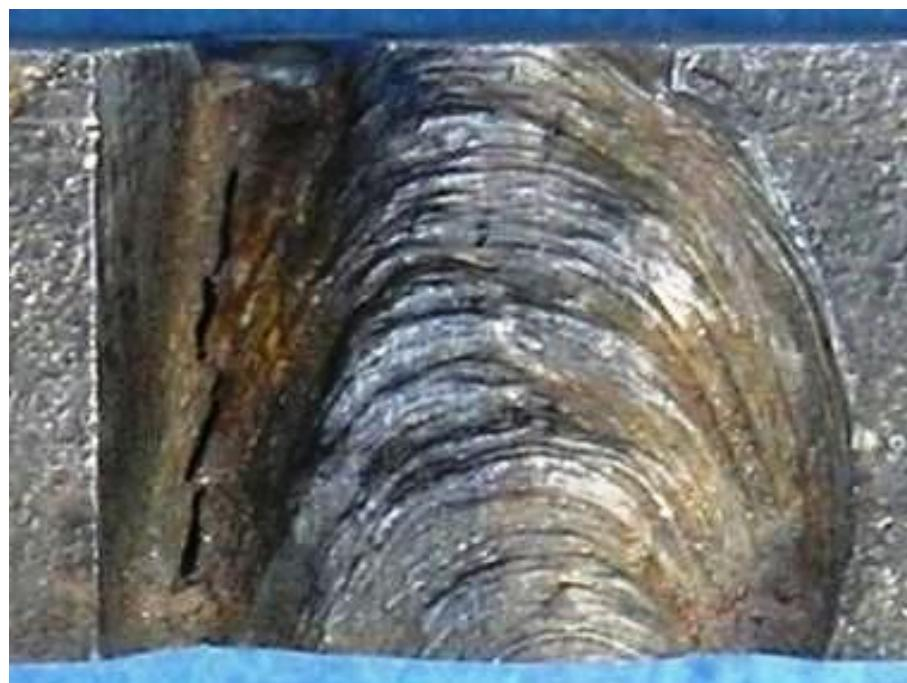
**Slika 4.2.5 Lice zavara uzorka 21 sa unosom topline 15 kJ/cm**
