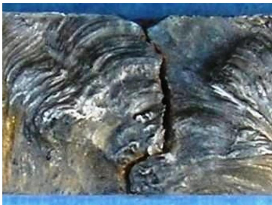
**Slika 4.2.9 Lice zavara uzorka 32 sa unosom topline 18 kJ/cm**
