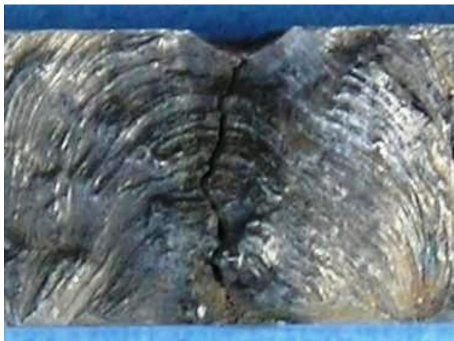
**Slika 4.2.11 Lice zavara uzorka 33 sa unosom topline 18 kJ/cm**
