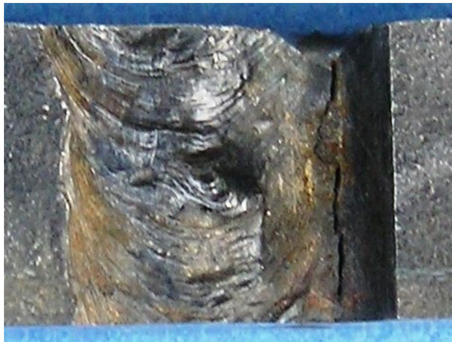
**Slika 4.2.7 Lice zavara uzorka 22 sa unosom topline 15 kJ/cm**
