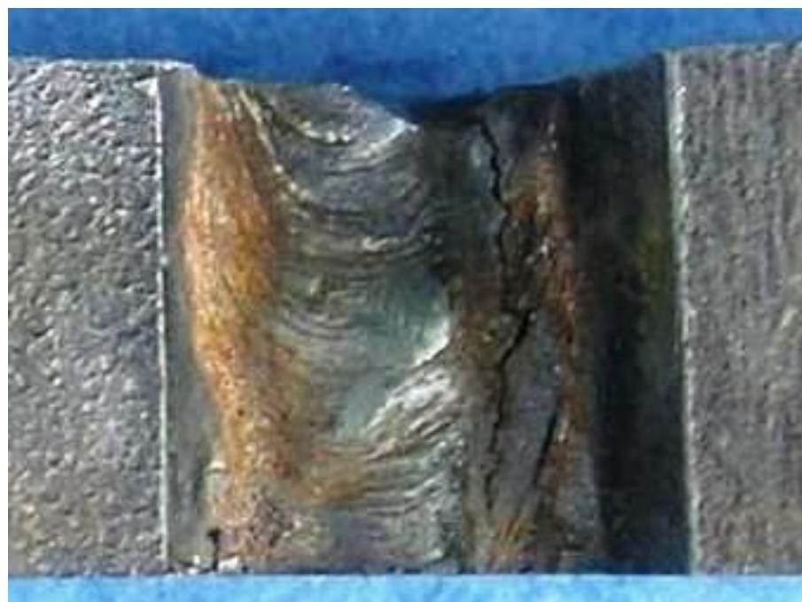
**Slika 4.2.3 Lice zavara uzorka 12 sa unosom topline 12 kJ/cm**
