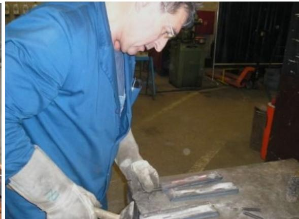
**Slika 3.5.14 Numeriranje i zacrtavanje iglom**
