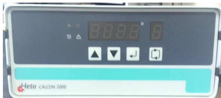
Slika 7. Calcon 2000 regulator temperature
