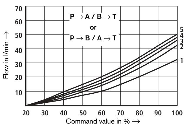
60 l/min nominal flow at 10 bar valve pressure differential
