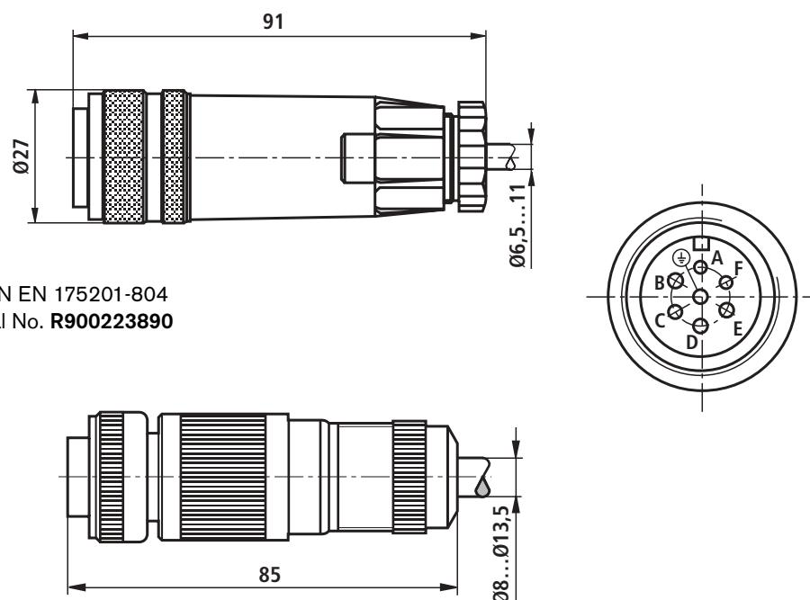
Plug-in connector to DIN EN 175201-804
