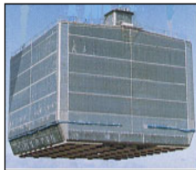
(IHI SPB Cargo Tank)
