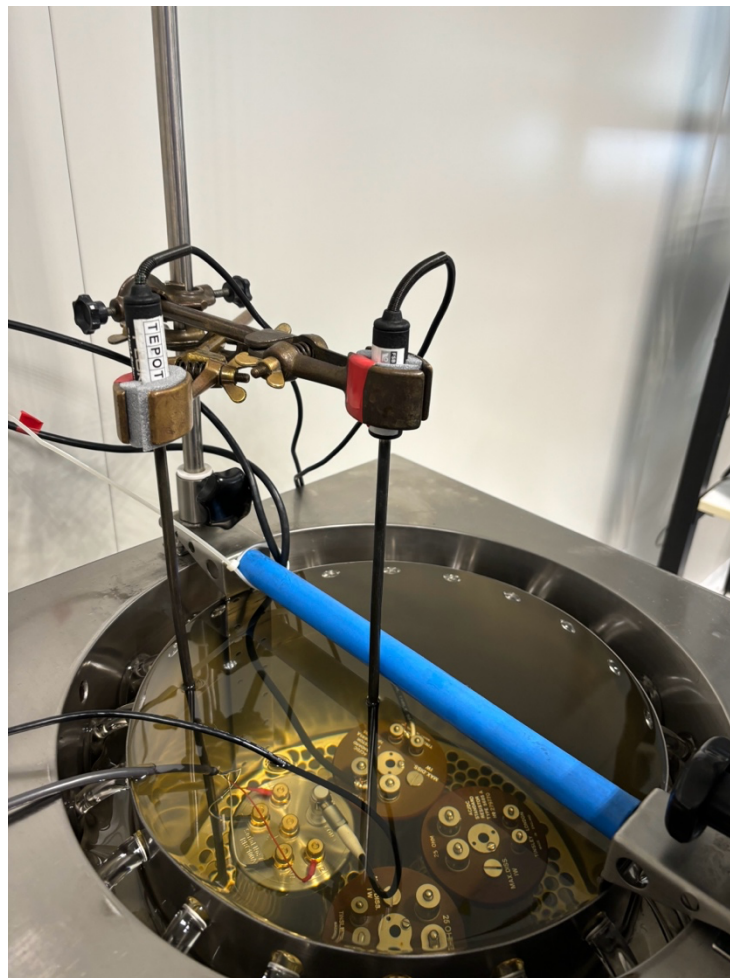
Slika 4. Raspored termometara i stalka u termostatiranoj kupki
