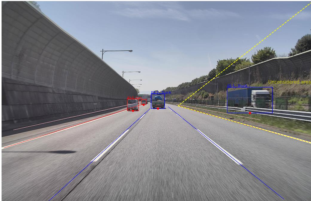
Figure 3.5: First polygon which filters out the irrelevant oncoming traffic objects (marked with yellow dashed lines).
