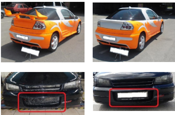
Figure 19: Improperly assembled rear spoiler with protruding parts and sharp edges (top left) and the appearance of the vehicle after removing of such spoiler to meet the test criteria (top right). A protective mesh
