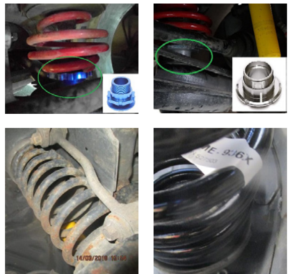
Figure 9: Improperly mounted suspension components (top left) and suspension components properly mounted by replacing the threaded nut which is compatible with the mounted spring (top right). Unauthorized mounting of used springs without identification codes (bottom left) and authorized mounting of new springs with identification codes (bottom right).
