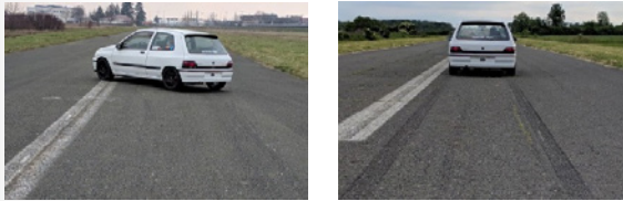
Figure 28: Stopped vehicle after braking at 80 km/h with defective brake system (left) and functioning brake system after the performed servicing (right).
