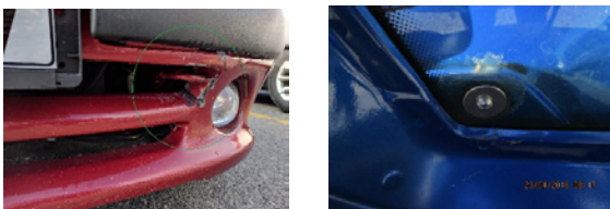
Figure 18: Cracked front bumper (left) and a roof spoiler improperly mounted by rear window drilling (right).
