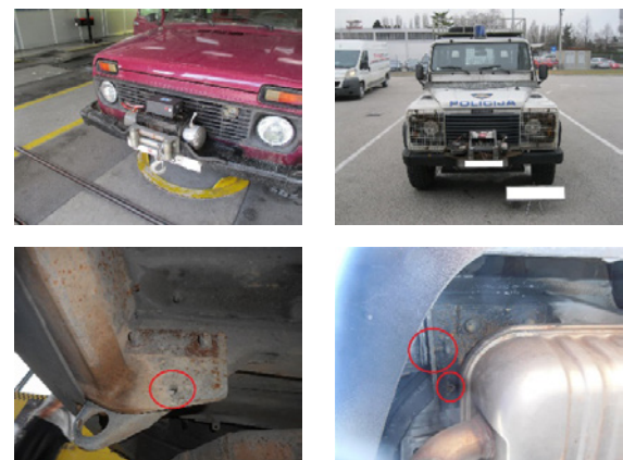
Figure 20: Improperly mounted winch protruding on the front bumper (top) and towbar holder improperly fastened onto the vehicle (bottom).
