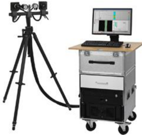
Figure 13. Optical measurement system Aramis 4M
