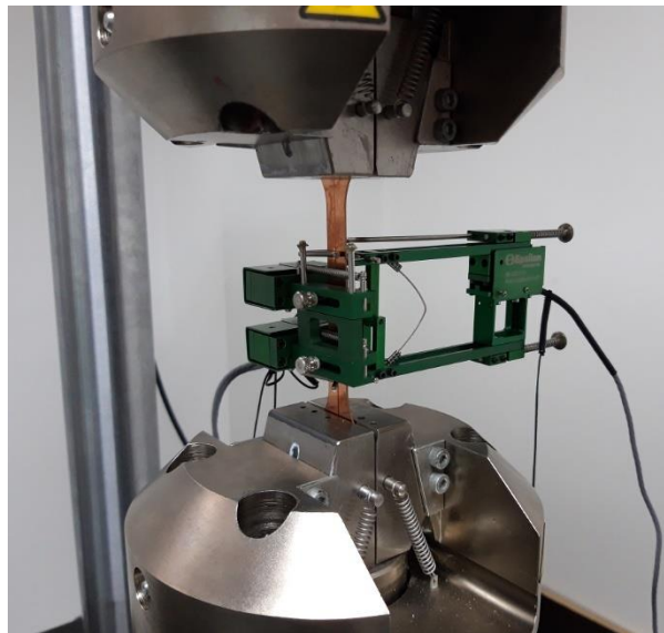
Figure 12. Tensile test specimen with longitudinal and lateral clip-on extensometer
