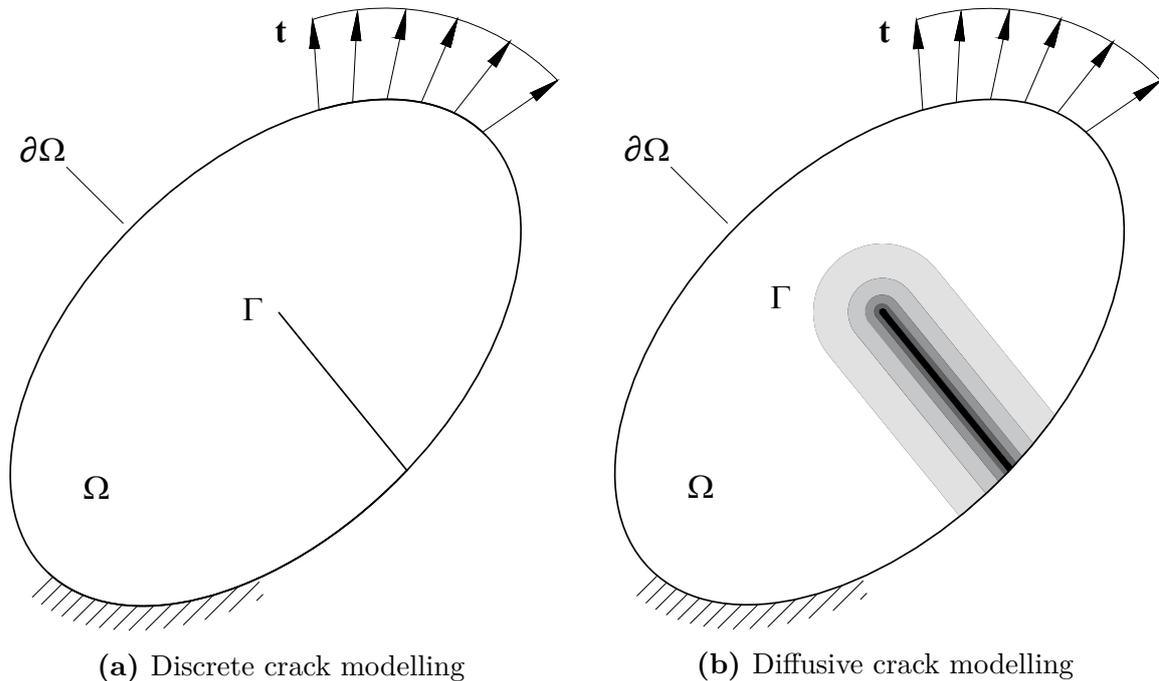
**Figure 1.3:** Schematic representation of the crack modelling approaches
