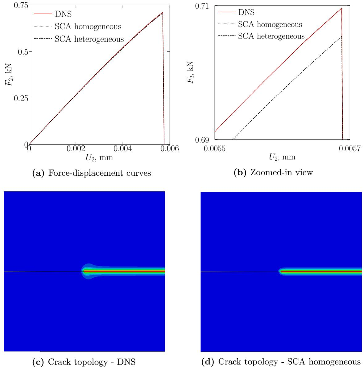
**Figure 4.16:** A 2D single-edge notched plate - tension test
