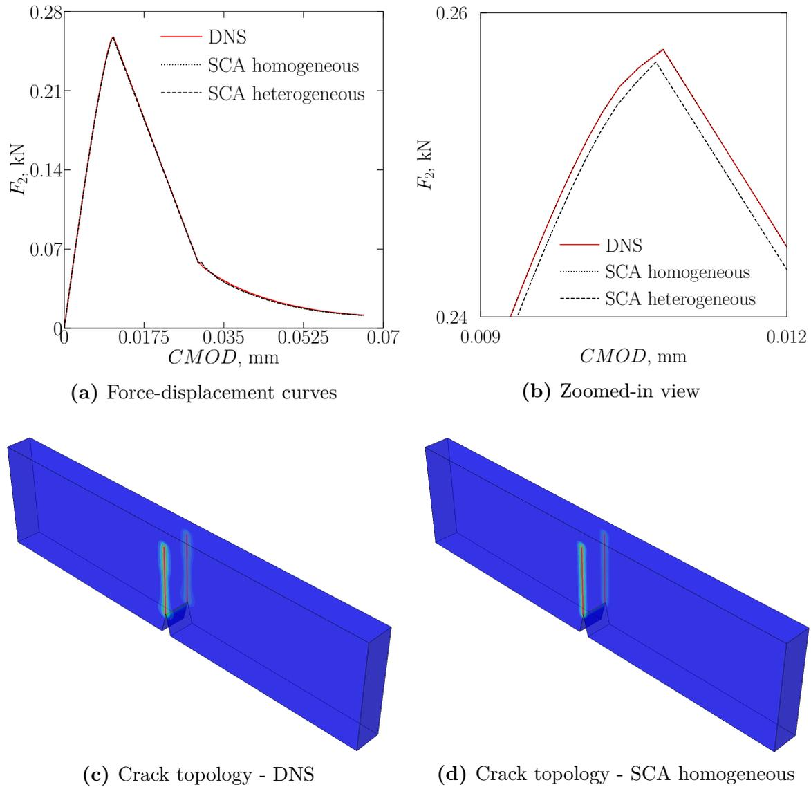
**Figure 4.23:** A 3D three-point bending specimen; volumetric-deviatoric split
