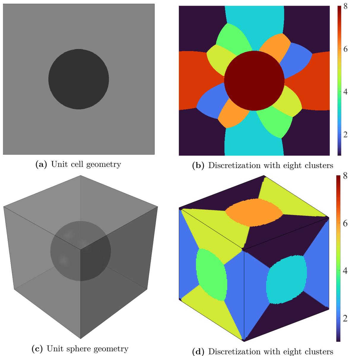
**Figure 2.1:** Microstructure decomposition into an appropriate number of material clusters
