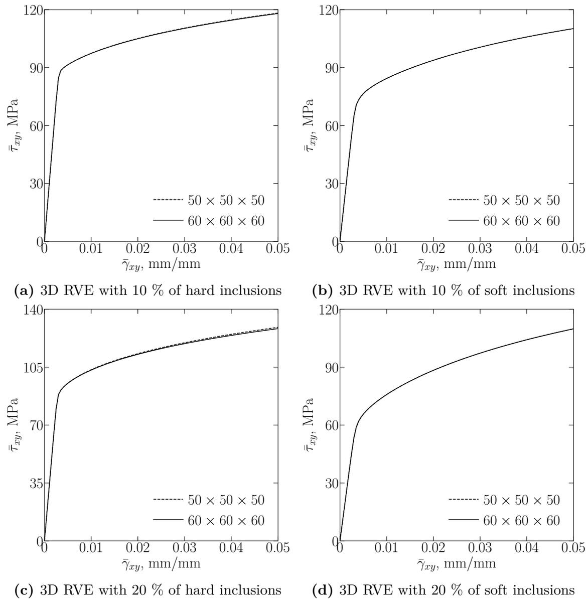
**Figure 2.26:** Influence of the finite element mesh discretization on the homogenized values for the case  $\bar{\epsilon} = \bar{\epsilon}^2$
