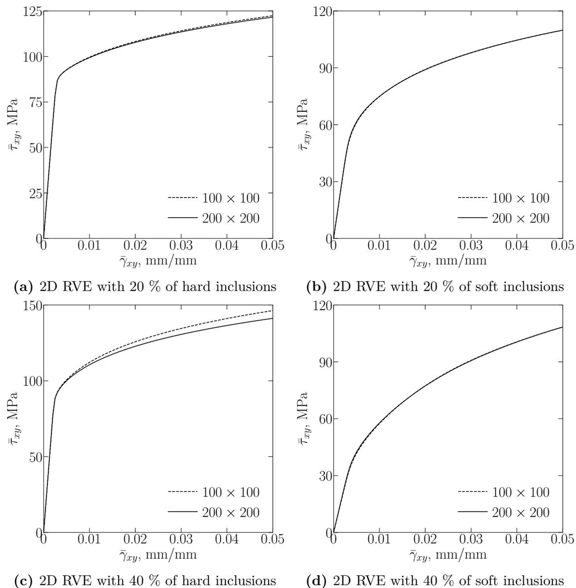
**Figure 2.12:** Influence of the finite element discretization on the homogenized values for the case of  $\bar{\epsilon} = \bar{\epsilon}^2$
