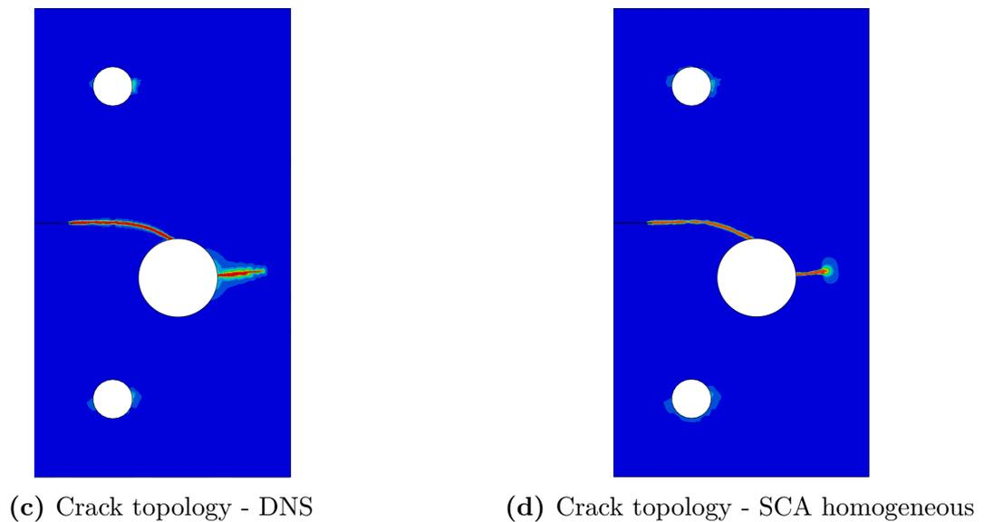
**Figure 4.20:** A 2D notched plate with a hole; spectral split
