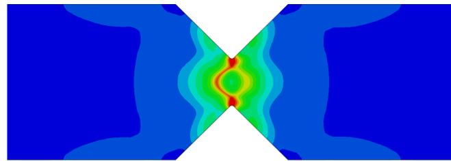
(c) Crack topology - DNS
