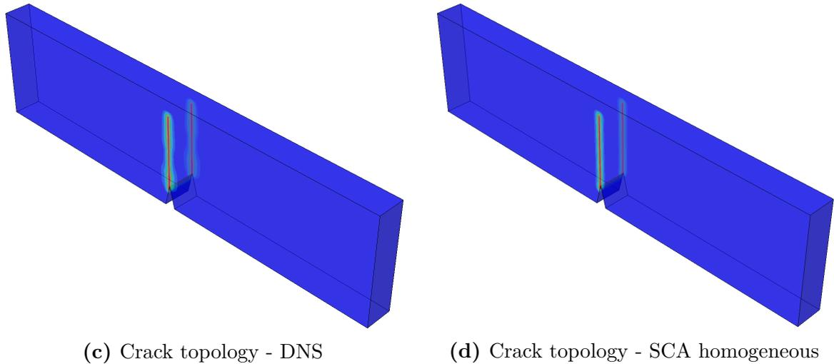
**Figure 4.24:** A 3D three-point bending specimen; spectral split
