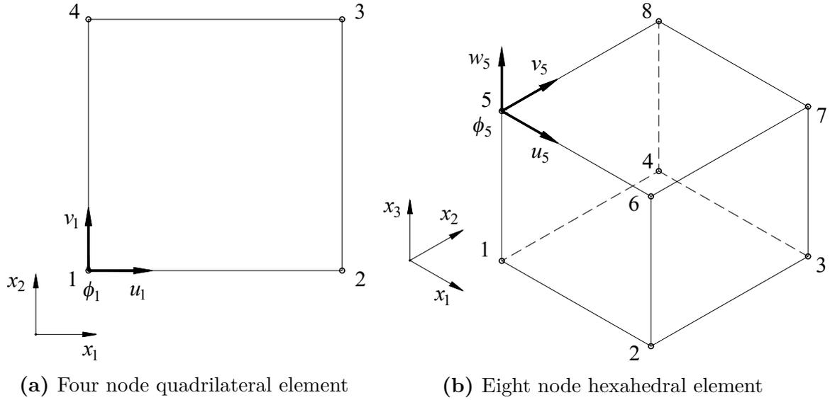
**Figure 3.5:** Implementation of the phase-field variable  $\phi$  into FEM
