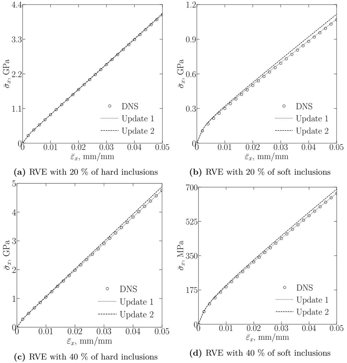
**Figure 2.17:** Comparisons of the homogenized stress-strain curves for a regression and projection based types of update for the case of  $\bar{\epsilon} = \bar{\epsilon}^{-1}$  and with 128 clusters
