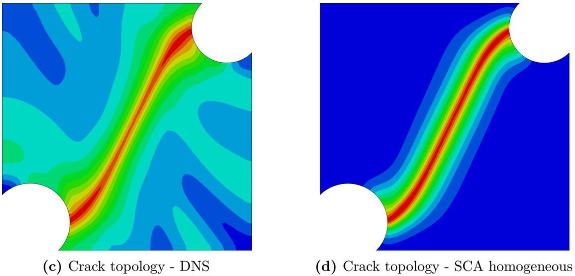
**Figure 4.29:** A 2D double-notched specimen (ductile fracture)
