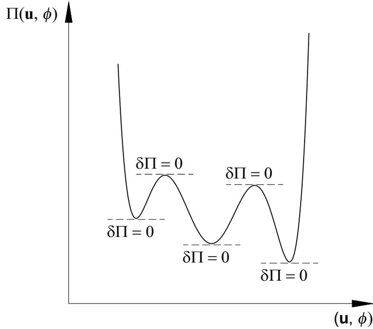
**Figure 1.4:** Schematic representation of non-convex energy functional
