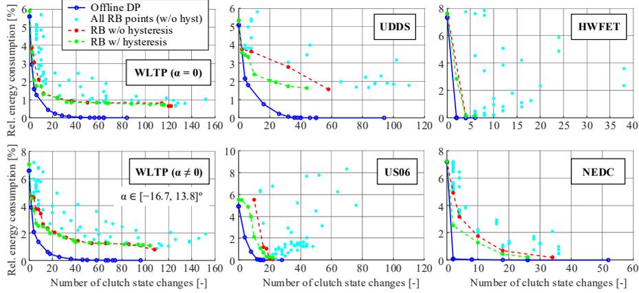
**Fig. 4.** Pareto optimal frontiers obtained by DP optimization, and RB control with and without hysteresis (a realistic non-zero road slope profile  $\alpha$  is optionally appended to WLTP cycle).
