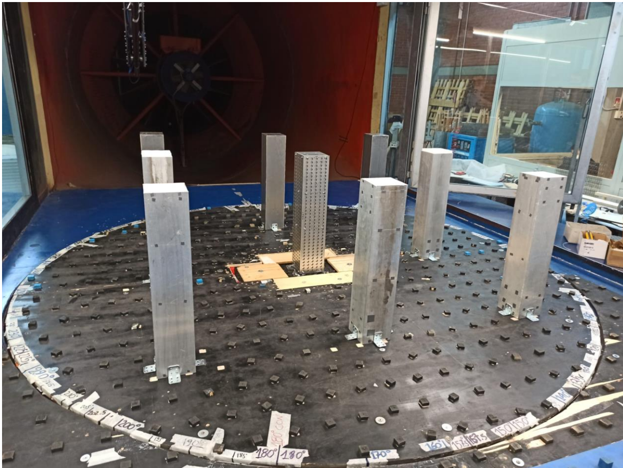
Figure 21. Arrangement of building models situated in the urban environment model
