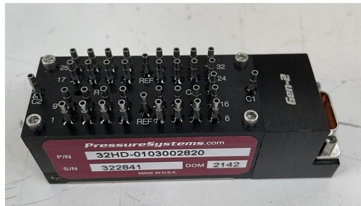
Figure 30. DTC pressure scanner
