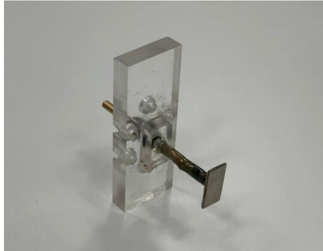
Figure 4. Smooth Ni electrode for Electrolyzer 4 on the electrode holder part
