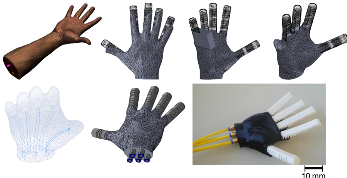
Figure 1: Anthropomorphic hand pre-processing and design: from initial model of a human hand to a finally printed and functional hand used for experimental verification.
