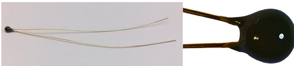
Slika 17 Termistor (NTC tip, bead in glass ) [13]
