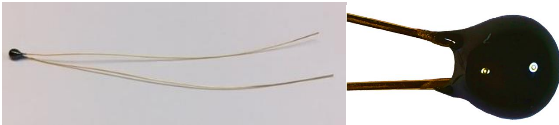
Slika 17 Termistor (NTC tip, bead in glass ) [13]
