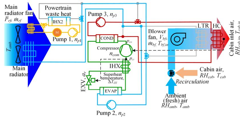
**Figure 1.** System schematic for heat pump (HP) mode.
