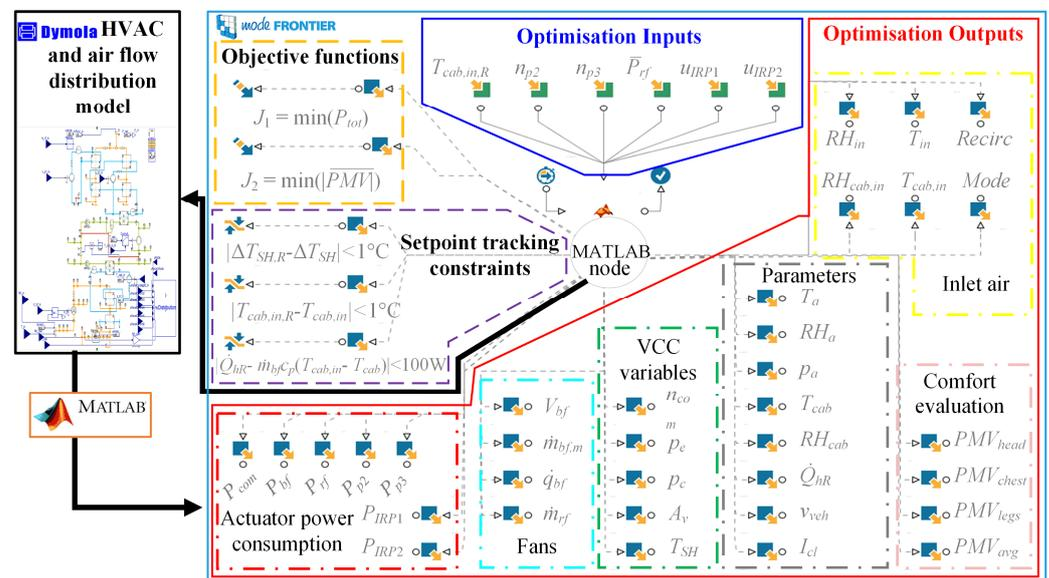
**Figure 4.** Optimisation framework implemented within ModeFrontier environment.
