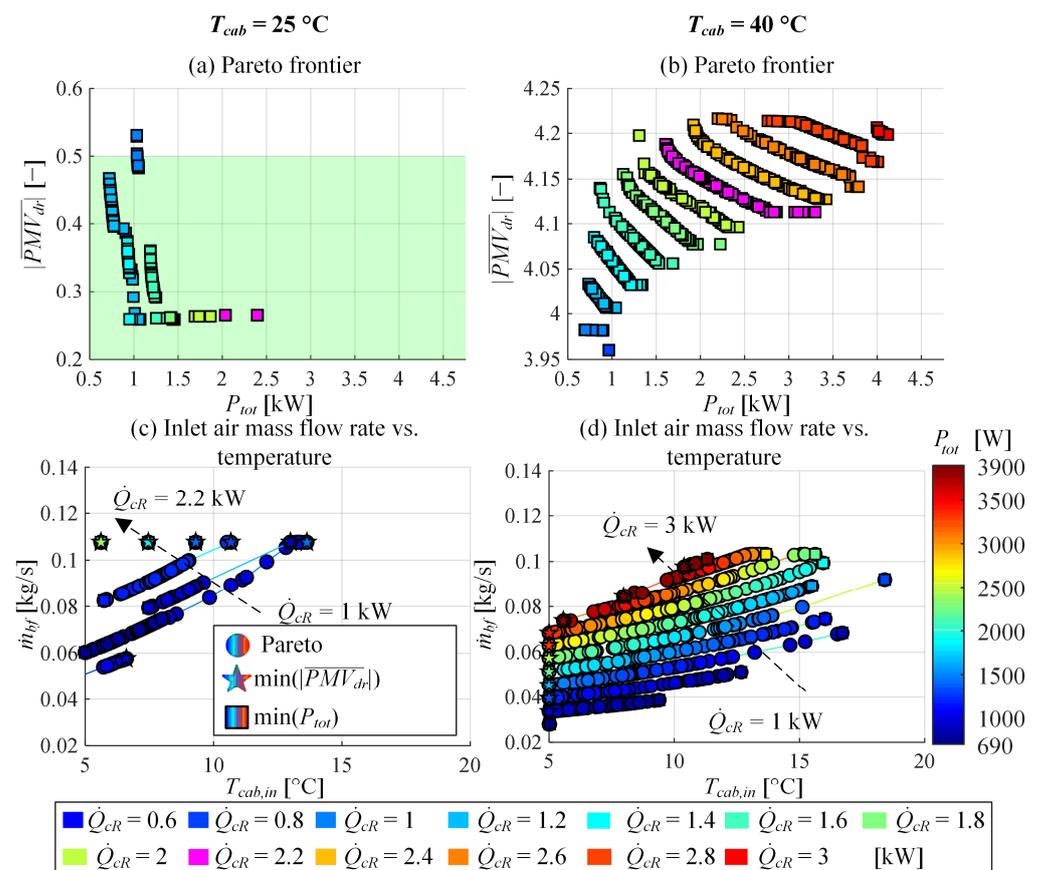
Figure A1. Multi-objective optimisation results for A/C mode.
