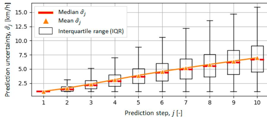
**Figure 14.** Boxplot of NN-DSTC model-predicted uncertainty parameter (i.e., standard deviation  $\hat{\sigma}_j$ ) of vehicle velocity prediction along steps  $j = 1, 2, \dots, H_p$  of prediction horizon.
