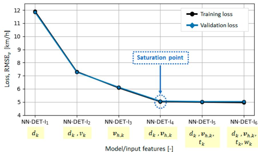
**Figure 5.**  $RMSE_v$  loss values obtained for each NN-DET-I<sub>n</sub> model (defined by characteristic input feature sets) by using training and validation datasets.
