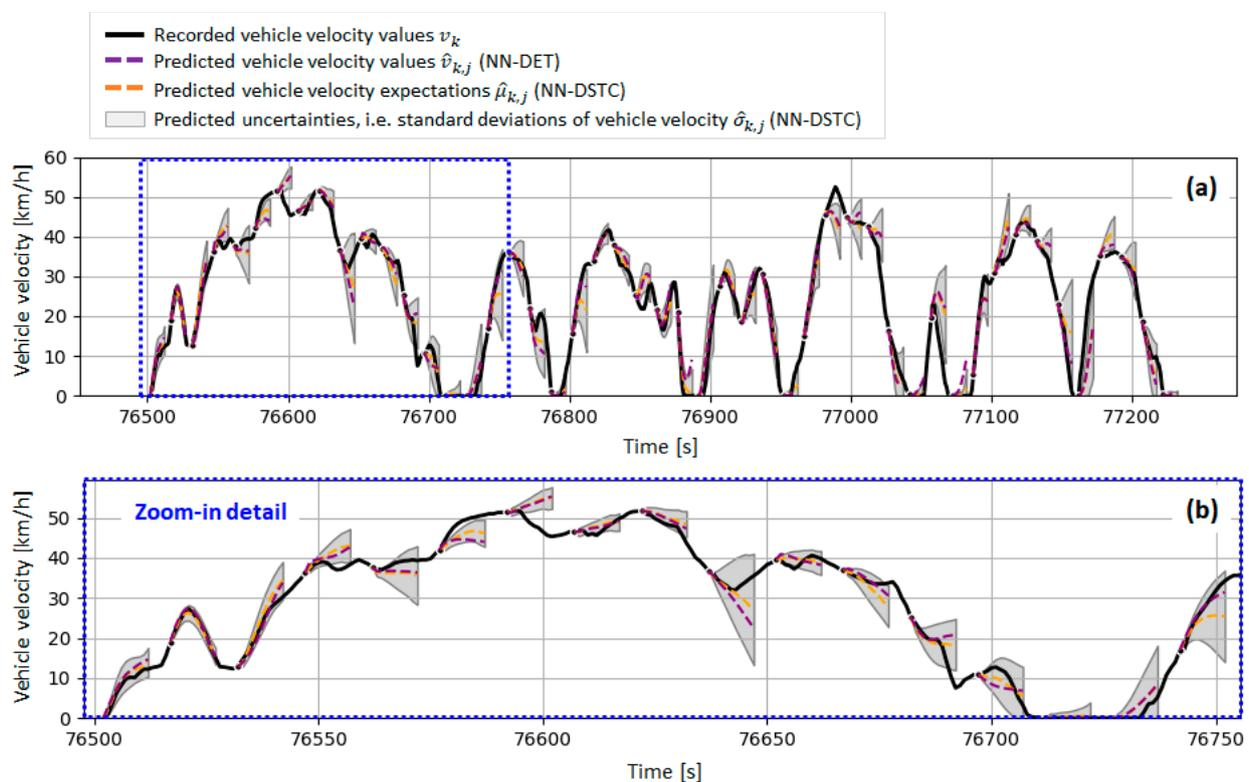
**Figure 13.** Comparative time response of vehicle velocity predictions provided by NN-DET and NN-DSTC models for one of driving cycles from test data set (a) and characteristic response zoom-in detail (b).
