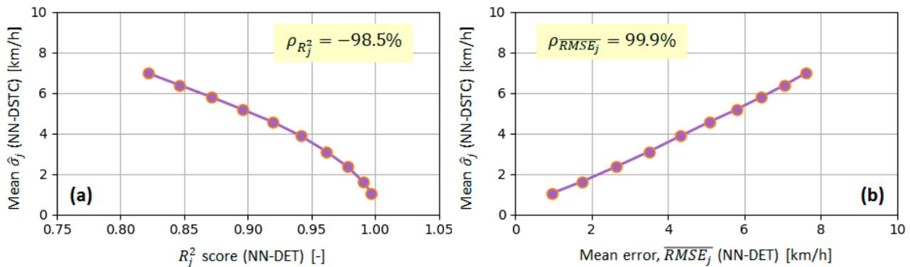
**Figure 15.** Dependence of NN-DET model velocity prediction accuracy metrics  $R_j^2$  (a) and  $\overline{RMSE}_j$  (b) on mean of NN-DTSC model-predicted standard deviation  $\hat{\sigma}_j$ , where  $\rho$  represents the corresponding Pearson correlation index value (100% means full correlation, and  $-100\%$  denotes full anti-correlation).
