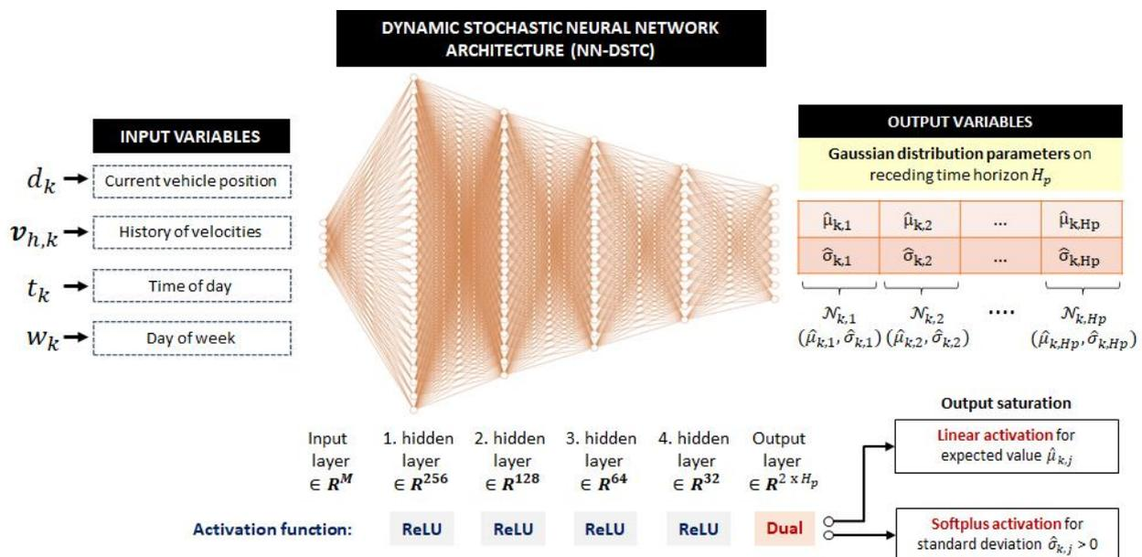
**Figure 9.** Proposed architecture of dynamic stochastic deep feedforward neural network (NN-DSTC) for predicting parameters of normal vehicle velocity distribution  $\mathcal{N}_{k,j}(\hat{\mu}_{k,j}, \hat{\sigma}_{k,j}); j = 1, 2, \dots, H_p$  along receding time horizon of length  $H_p$ .
