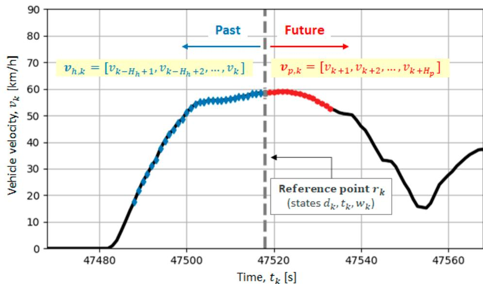
**Figure 3.** Illustration of the process of generating input-output datasets  $\mathcal{X}$  and  $\mathcal{Y}$ , necessary for training, validation, and testing of NN-based velocity prediction models.
