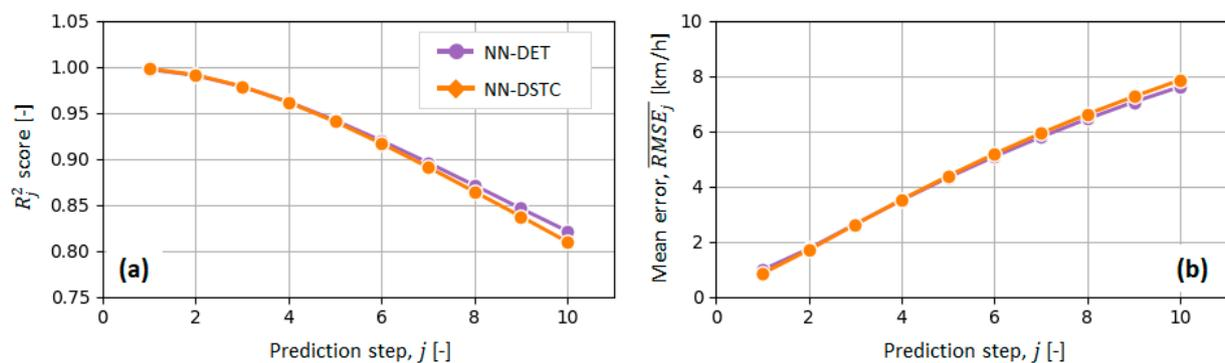
**Figure 12.** Comparative plots of prediction performance of NN-DET and NN-DSTC models, expressed in terms of  $R_j^2$  (a) and  $\overline{RMSE}_j$  (b) metrics, determined for different prediction steps  $j$  along prediction horizon  $H_p$ .
