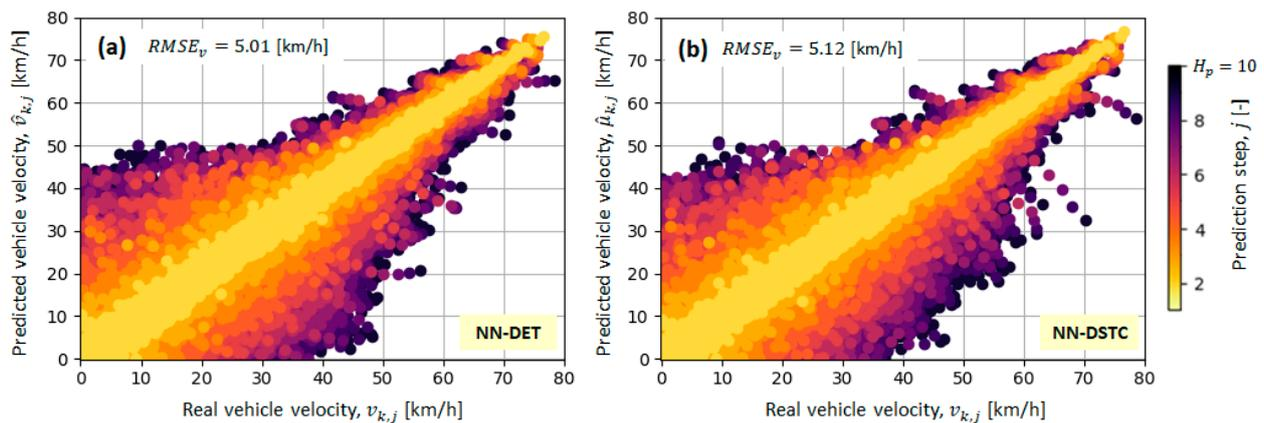
**Figure 11.** Predicted velocity  $\hat{v}_{k,j}$  and velocity expectation  $\hat{\mu}_{k,j}$  in relation to real velocity values  $v_{k,j}$  for NN-DET model (a) and NN-DSTC model (b), respectively, where predictions for each  $j$ th time step along the prediction horizon  $H_p$  are marked in different colours.
