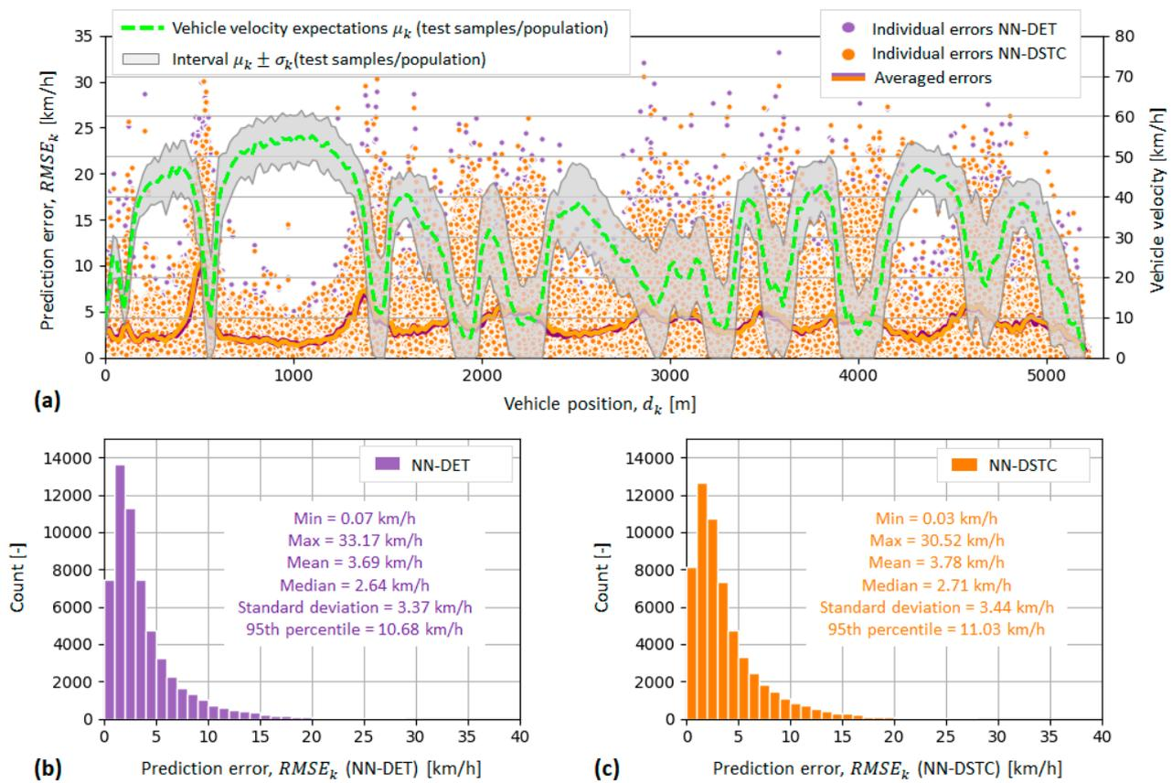
**Figure 16.** Scattering of NN-DET and NN-DSTC models individual RMS velocity prediction errors along the selected bus route (a), including the corresponding distributions given separately for NN-DET (b) and NN-DSTC models (c).
