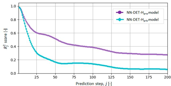
**Figure 8.**  $R^2_j$  score values corresponding to  $j$ th discrete step of prediction horizon with length  $H_p = 200$  s and calculated for validation data set (note that for given sampling time of 1 s, the prediction in-interval of, e.g.,  $j = 200$  steps correspond to the length of 200 s).
