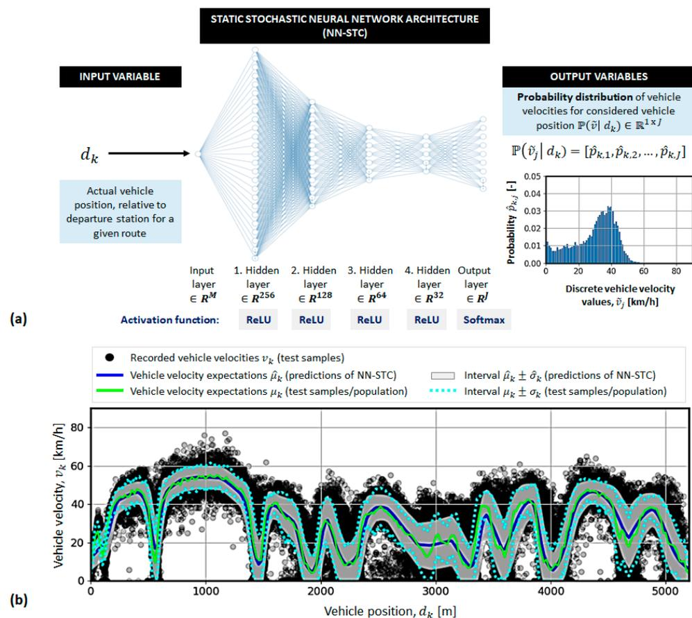
**Figure 1.** Illustration of previously proposed static stochastic neural network (NN-STC) model [22] for predicting city bus velocity distribution along route (a), including related testing results (b).
