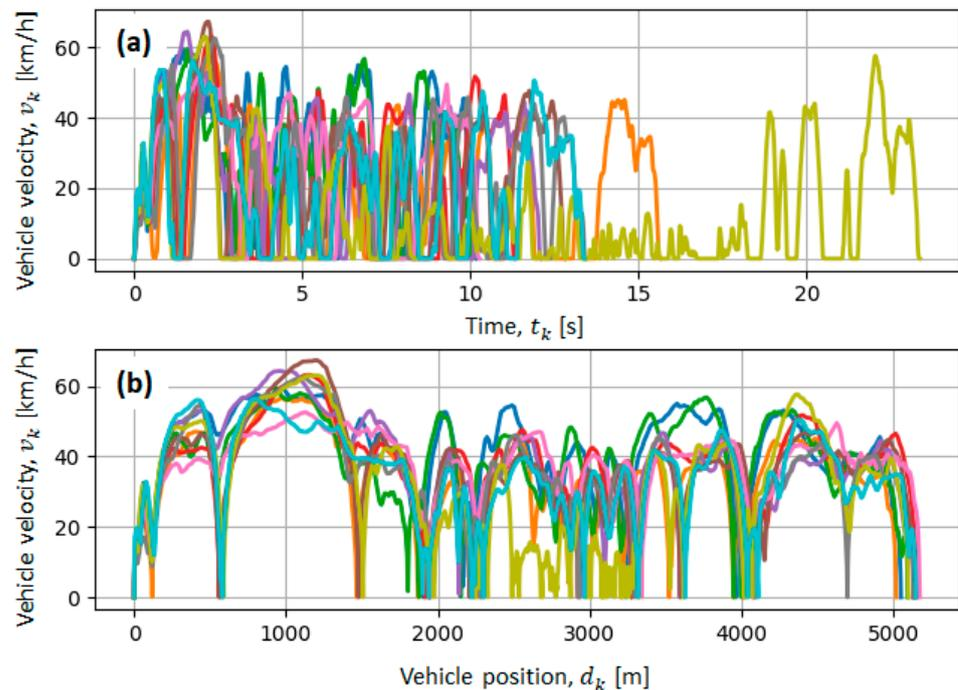
**Figure 2.** Examples of ten randomly selected valid recorded driving cycles for the direction Babin kuk–Pile: velocity vs. time (a) and velocity vs. travelled distance (b) profiles.
